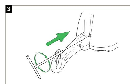
Insert the special tool into the opening. Turn it clockwise to lower the patient. The tool rotates the motor directly, so each turn of the tool will slightly lower the patient.
