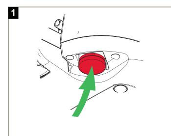
Press on the red emergency shut-off button under the lift. Move the lift with the patient over the bed or the wheelchair.
